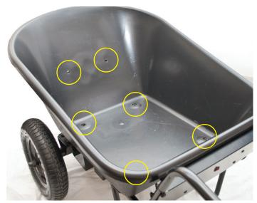
2. Insert M8 x 25mm carriage bolts (U) through all six bolt holes of tray. These will extend through the tray brace (two) and frame (four). Secure all six with M8 hex nuts (T). Tighten all nuts with a wrench.
