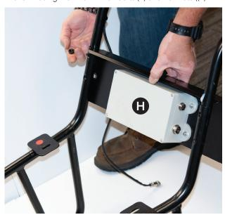
5. Match up wires to their ports and plug in; twist threaded couplers to secure.
