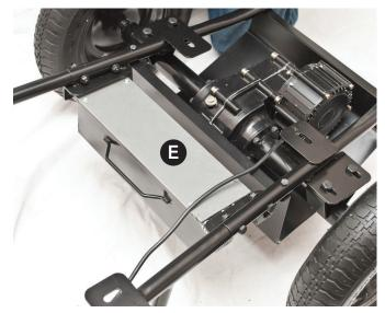
$\bf 3$ . Insert power cord plug into outlet on the right side of the battery box. Push in to secure.
