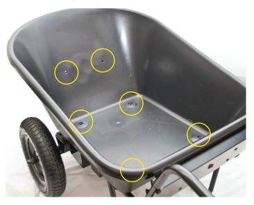
2. Insert M8 x 25mm carriage bolts (U) through all six bolt holes of tray. These will extend through the tray brace (two) and frame (four). Secure all six with M8 hex nuts (T). Tighten all nuts with a wrench.
