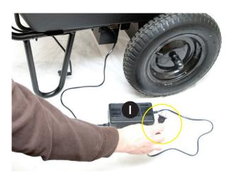
2. Remove power plug from battery box (E) located on the right side of box.
