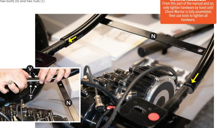
2. Attach right (K) and left (J) legs to the other side of the assembled axle frame mounts. Secure with M8 x 40mm hex bolts (V) and hex nuts (T).
