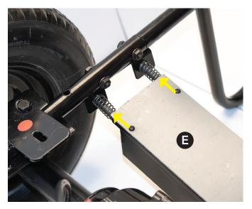
2. Push the battery box to the right to compress springs, then lift left side up and insert into left side mounts as shown. Release. The box should now be suspended between the frame.
