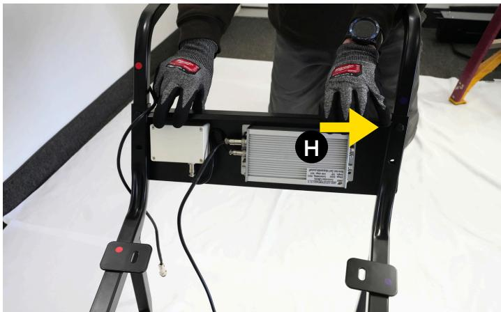
4. Attach the right side of electronics box to right handle as shown using M8 x 40mm hex bolts (V) and hex nuts (T).
