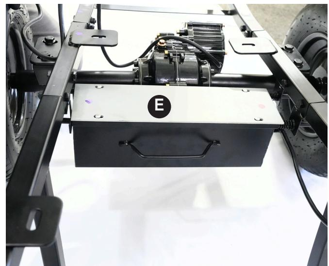
3. Insert power cord plug into outlet on the right side of the battery box. Push in to secure.
