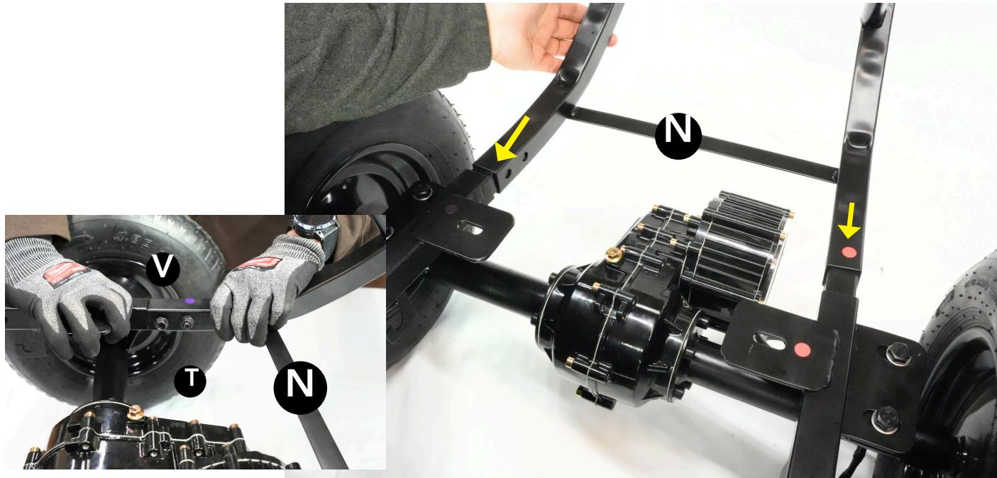
2. Attach right (K) and left (J) legs to the other side of the assembled axle frame mounts. Secure with M8 x 40mm hex bolts (V) and hex nuts (T).
