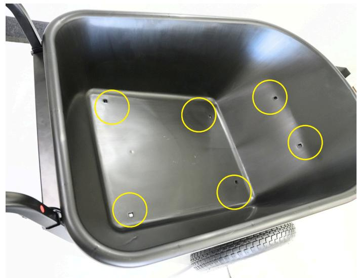
2. Insert M8 x 25mm carriage bolts (U) and provided washers through all six bolt holes of tray. These will extend through the tray brace (two) and frame (four). Secure all six bolts with M8 hex nuts (T). Tighten all nuts with tools.
