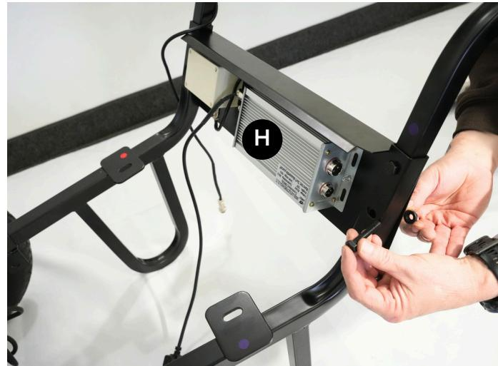
5. Match up wires to their ports and plug in; twist threaded couplers to secure.
