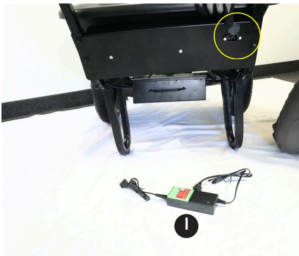
2. Remove power plug from battery box (E) located on the right side of box.
