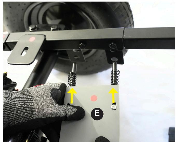
2. Push the battery box to the right to compress springs, then lift left side up and insert into left side mounts as shown and release. The box should now be suspended between the frame.
